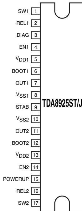
Figure 9-42 Internal block diagram and pin configuration
